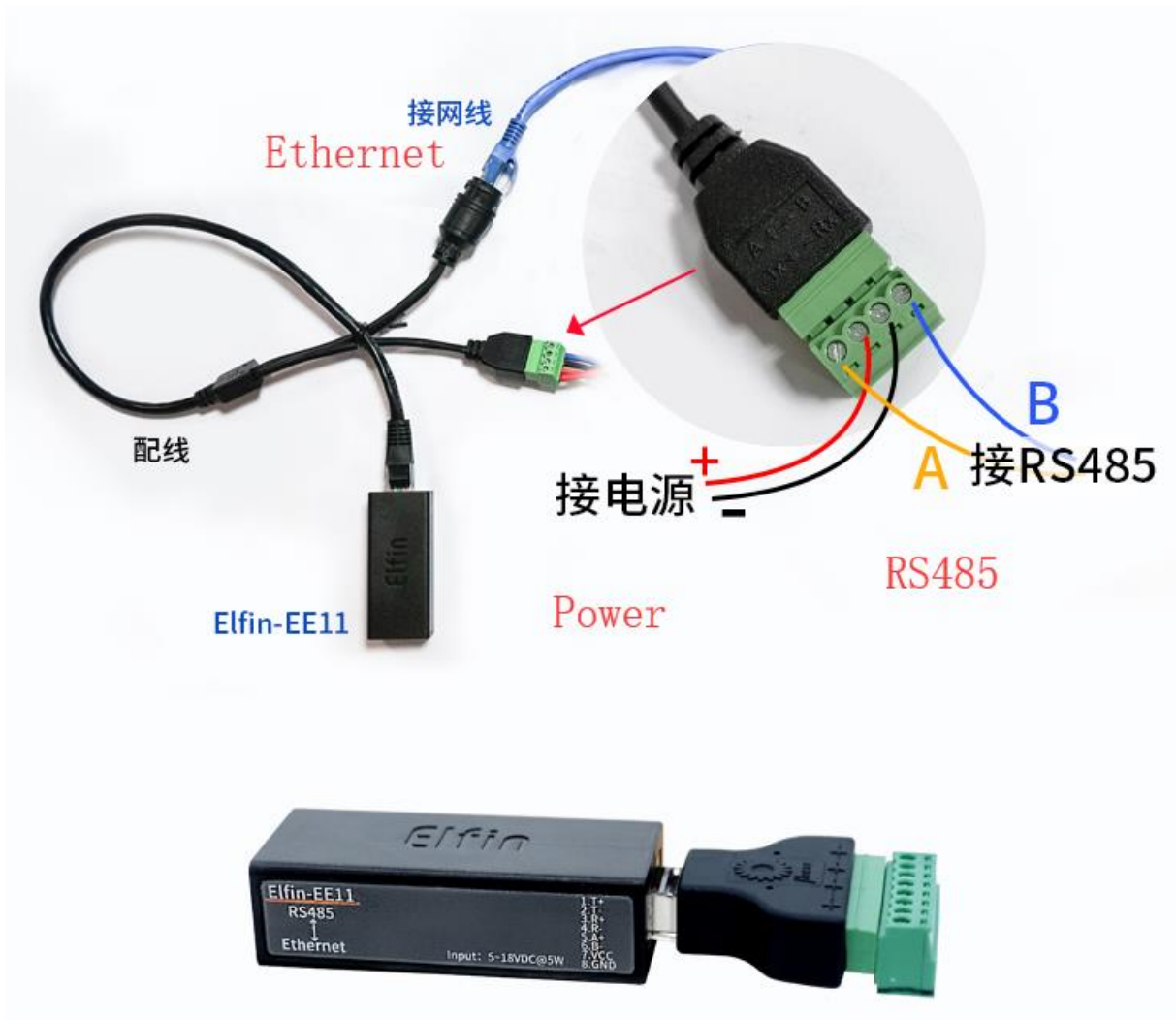
Figure 11. Interface Conversion Cable
