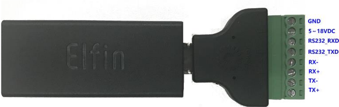
Figure 7. EE10 +8PIN Connector
