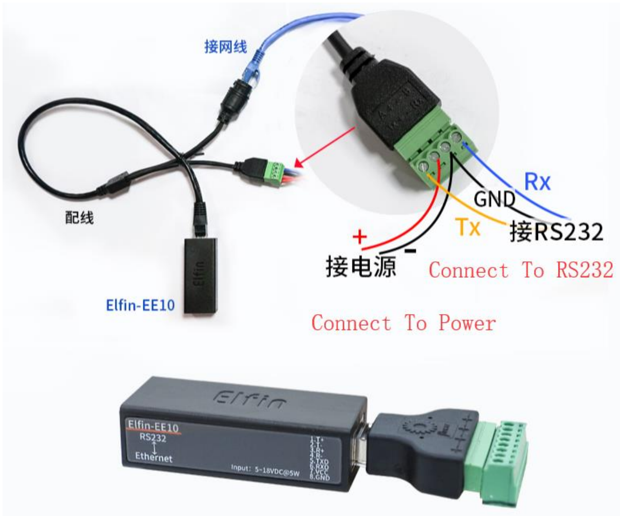
Figure 9. Interface Conversion Cable
