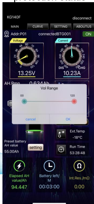
Figure 3-5-58 Voltage scale range
