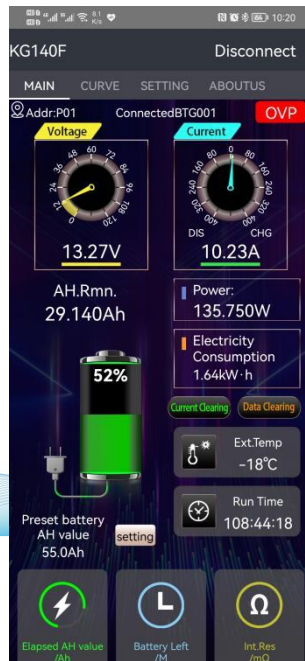
Figure 3-5-12 Over-voltage protection status
