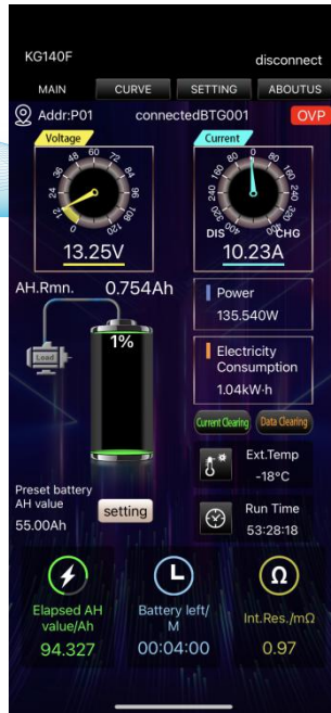
Figure 3-5-55 Over-voltage protection status
