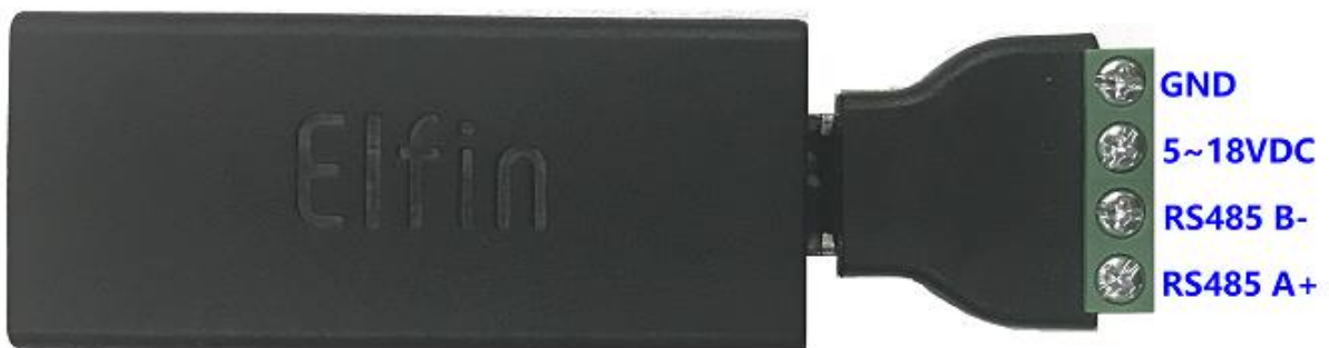
Figure 11. EW11+4PIN Connector
