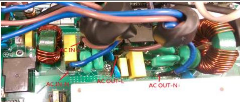
Remove AC SPS cable and MPPT power supply cables.
