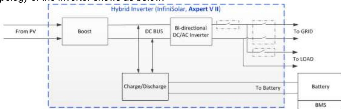
Compare with UPS or normal inverter, INVERTER combines a solar charger inside. Solar charger can be a supplement for battery when there is not grid or for saving energy purpose. And with the solar charger, the inverter can have more working modes than UPS. For detail information please refer to our user manual.
