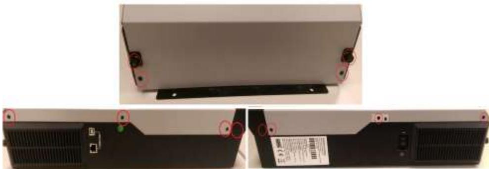
Remove LED cable and LCD cable, and take out the top cover.
