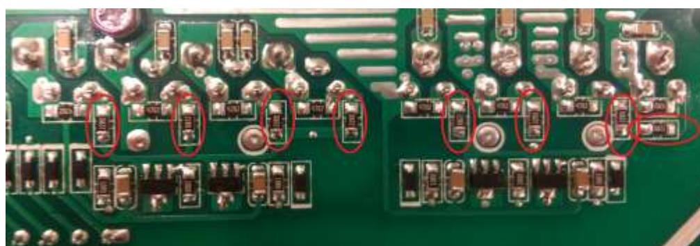
Use multimeter to measure each resistor, find the burnt resistors and replace them; don't need to replace them all.
