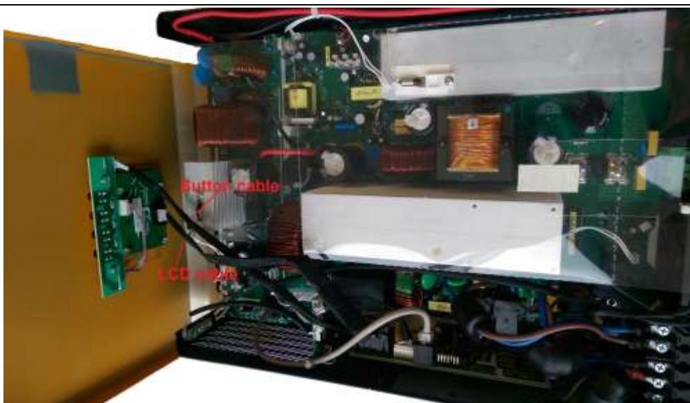
Remove comm cable and MPPT Comm cable and Anti dust cable and screw, and take out comm board.
