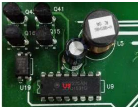
The U9 is (IC PWM CNTL SG3525ANG DIP-16)
