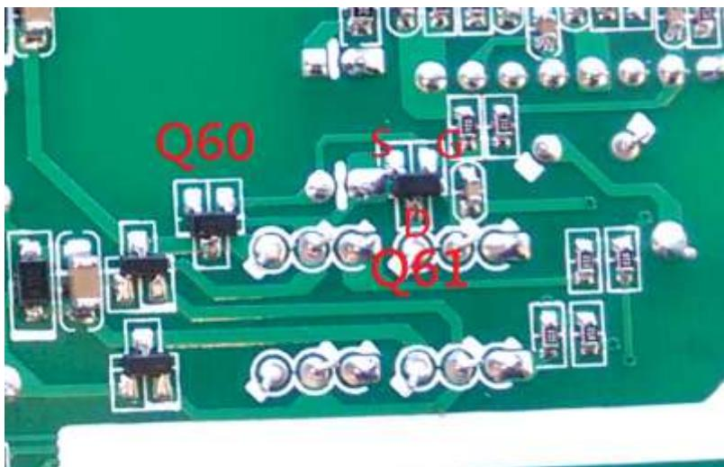
The Q60 and Q61 the MOSFET are (UT3404G 5.8A 30V SOT-23)
