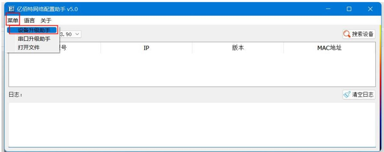
Step 3: In the pop-up "Device Network Upgrade Assistant" dialog box, click "Search Device" (the computer and device should be in the same network segment), and click "Stop Search" after finding the device;
