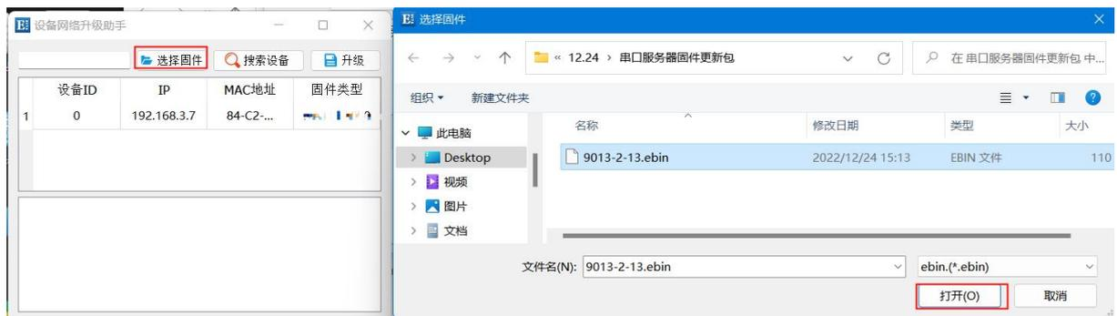
Step 5: Select the equipment to be upgraded, click "Upgrade", the progress bar will start to change, and wait for the upgrade to complete.
