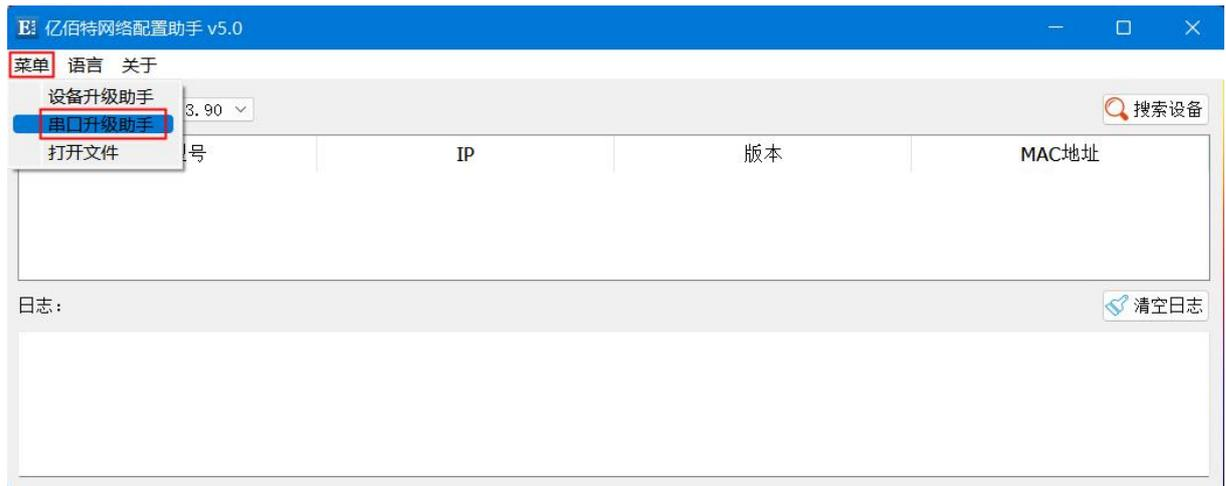
Step 3: First connect the USB port of the computer, select the corresponding port number in the pop-up "Serial Port Upgrade Assistant" dialog box, and click "Open Serial Port";
