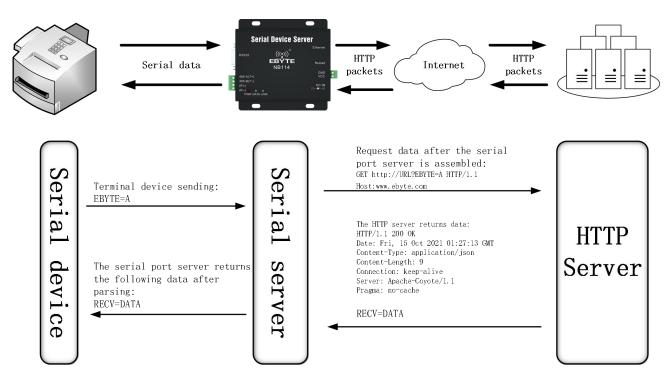
Configure the local network parameters and the HTTP server address and port(You are advised to enable DHCP and random ports), As shown in the figure below(Above is the upper computer, below is the web page):
