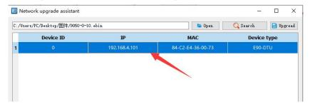
Step 4: Click to start the upgrade, the device indicator flashes, and wait for the upgrade to complete.
