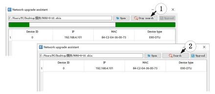
Step 3: Select the corresponding device that needs to be upgraded;
