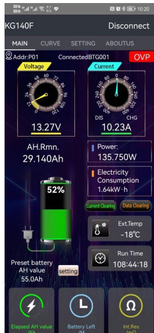
Figure 3-5-12 Over-voltage protection status
