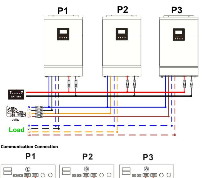
**WARNING:** Do not connect the current sharing cable between the inverters which are in different phases. Otherwise, it may damage the inverters.
